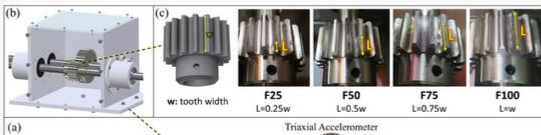
Figure 4. The experimental set-up: (a) photo of the gearbox including the sensors (accelerometer and tachometer) locations, (b) cross-sectional view of the one-stage gearbox and (c) the pinion single-tooth fault scenarios F25, F50, F75 and F100.
